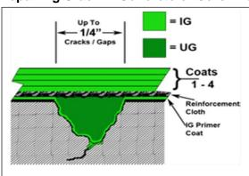
Repairs should be made with an application of Liquid Rubber™ IG as a primer followed by an embedded reinforcement fabric, fabric needs to be at least 4" in width, with 2" each direction from repair at all open joints, seams, cracks, holes, or areas of damage as well as at all penetrations, inside or outside corners and at any pan, or threshold that are determined by specification to be part of the waterproof envelope.
